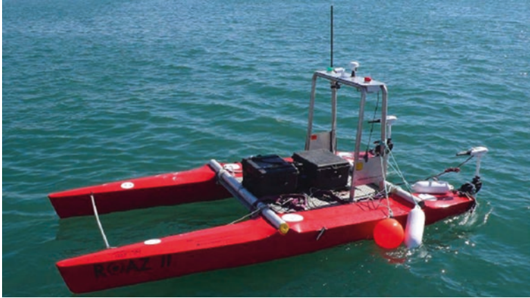
Fig. 4.2 The ROAZ II (2007), an example of ASV [3]
