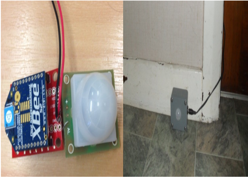
Fig. 3.10 Fabricated Wireless PIR (motion) Sensing Systems
