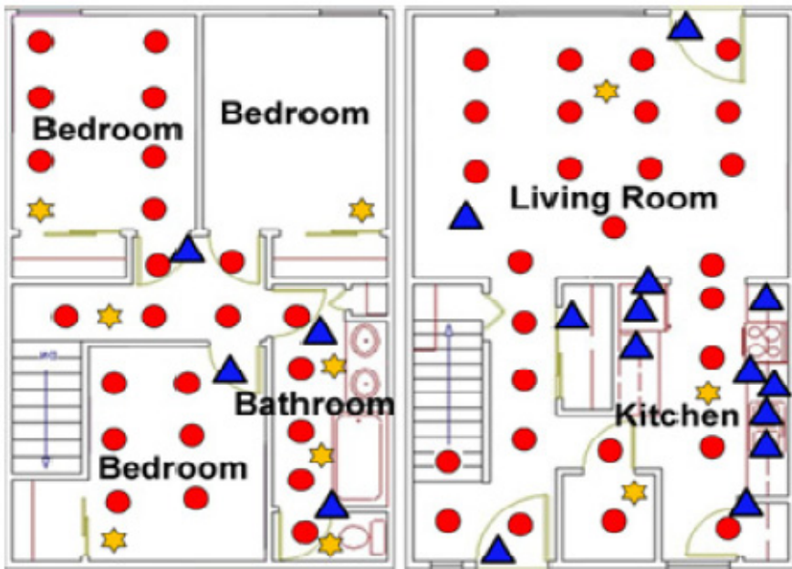
Fig. 2.5 One of the Test-Bed Sensor Installation of CASAS Project (Rashidi & Cook, 2011) (Rashidi & Cook, 2011)
