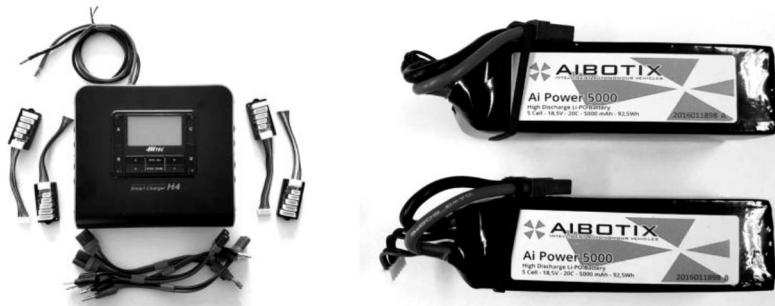
FIGURE 2.23 (a) Multicharger, and (b) Two batteries of UAV.
