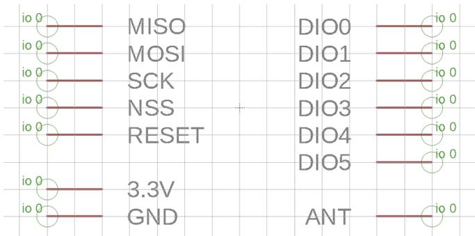
**FIGURE 4-3:** Adding pins. Group pins functionally in the schematic symbol. In this case, all the module's IO pins are together on the right, the SPI communication interface is on the left, and power and the antenna are at the bottom.
