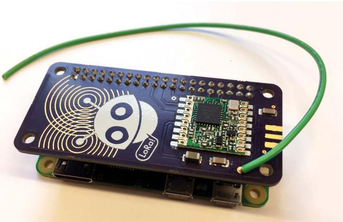
**FIGURE 4-1:** The finished board, with custom artwork on the silkscreen layer and the top solder mask layer, as described in this chapter
