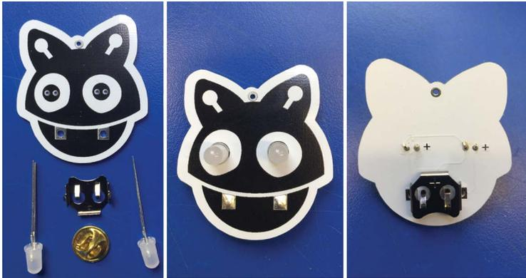
**FIGURE 2-1:** A successfully soldered blinky badge board. These RGB LEDs have a forward voltage of about 3V and slowly cycle through different colors.
