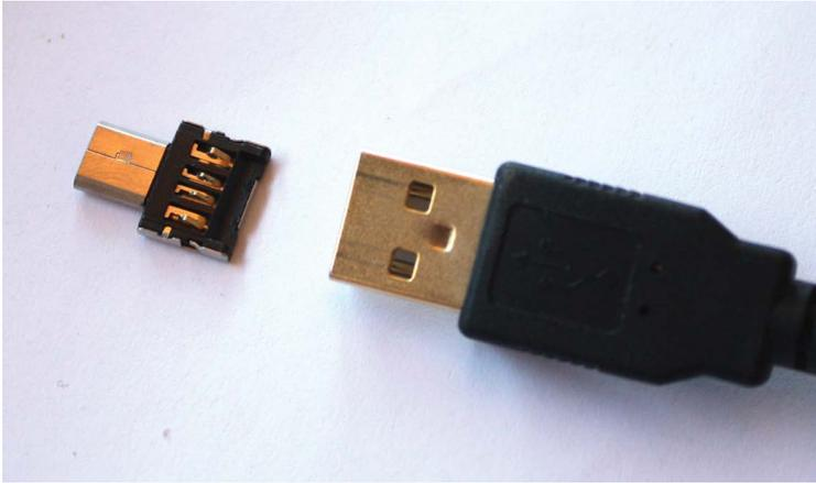
**FIGURE 1.6:** A USB On-the-Go (OTG) adapter
