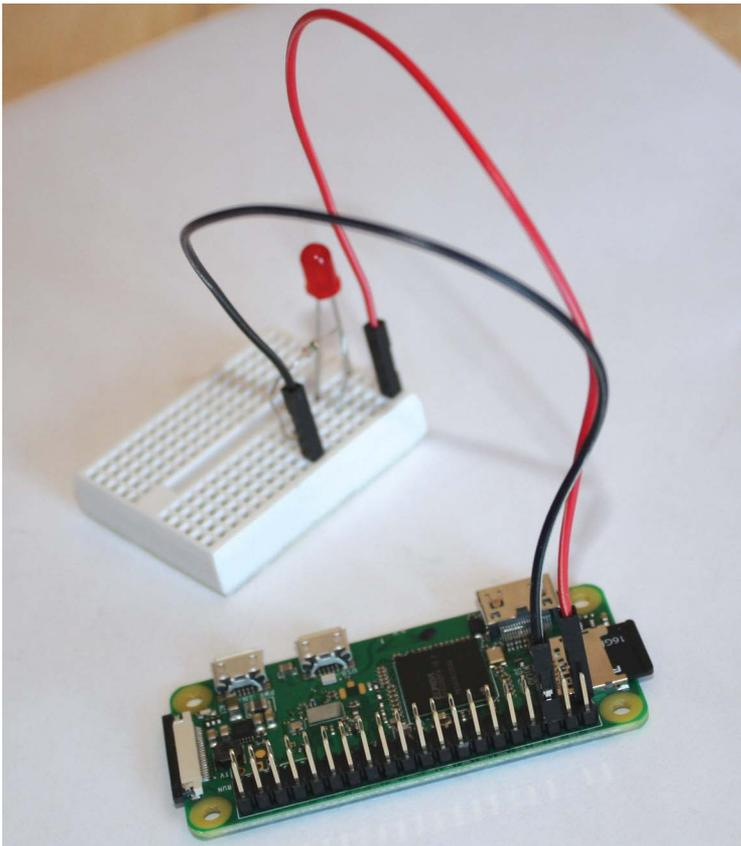
**FIGURE 2.2:** Male header with female-to-male leads
