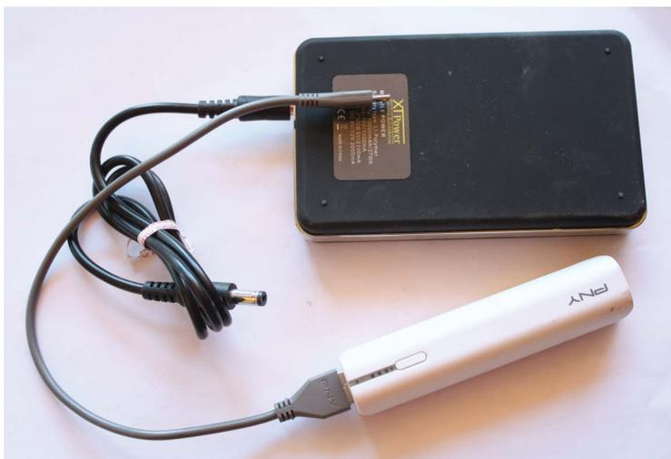
**FIGURE 4.13:** A couple of portable USB chargers
