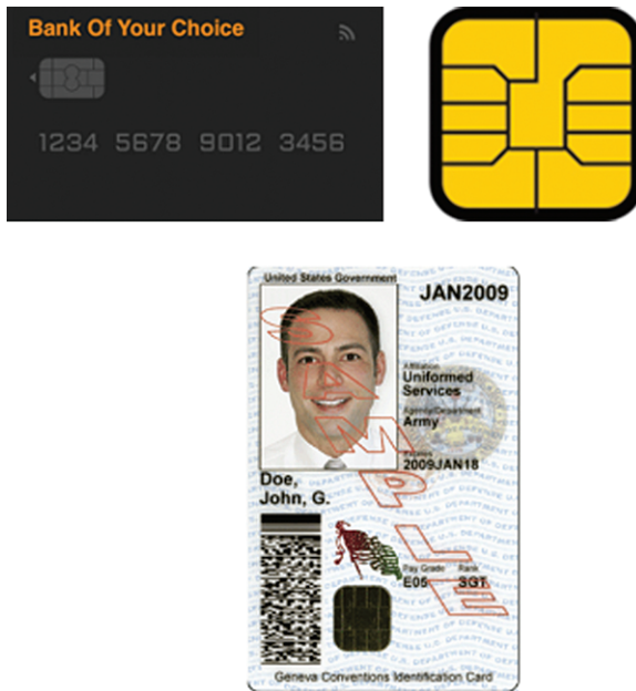
Figure 7-10 An Access Card with a Chip and the Chip's Inside Details (U.S. Government and a Typical Credit Card)
