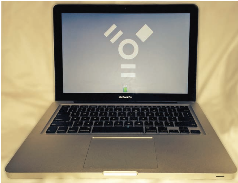
FIGURE 12.14 Target Disk Mode (TDM) on a MacBook Pro
