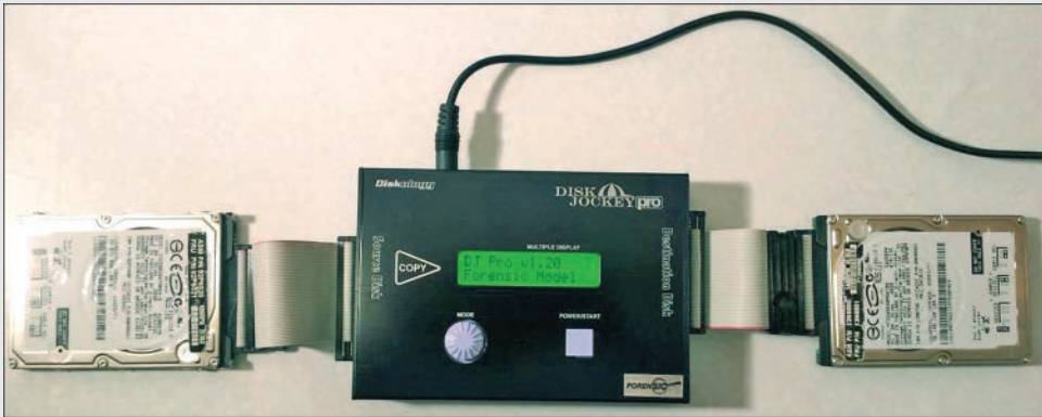
FIGURE 3.11 Configuration of hard drives connected to the Disk Jockey PRO
