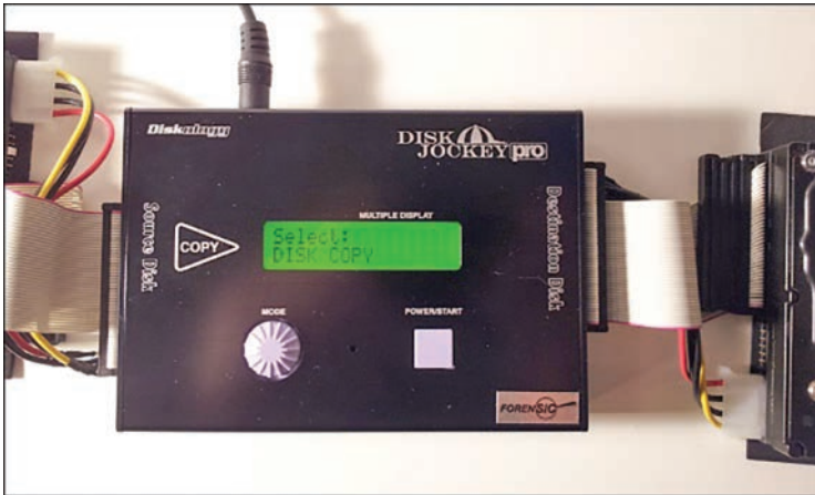
FIGURE 3.10 Cloning a hard disk drive with Disk Jockey PRO Forensic Edition
